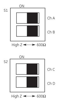
The A8920A units are shipped with the input impedance set at (high-Z). To select a  $600\Omega$  input impedance in place of the high-Z input, set switches SW1 and SW2 on the audio to  $600\Omega$ .
